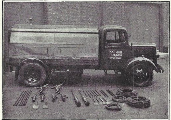
FIG. 1.—SELF-MOBILE AIR-COMPRESSOR AND TOOL EQUIPMENT.
