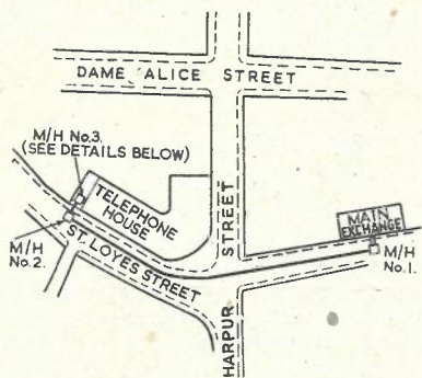
ROUTE OF EXTERNAL DUCT TRACK.
