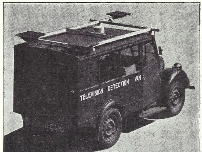
FIG. 2.—THE DETECTION VAN, SHOWING LOOP AERIALS ON ROOF.
