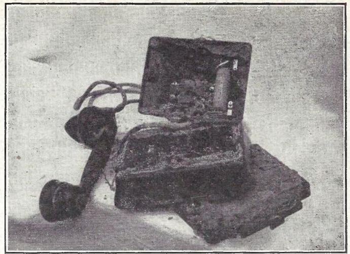
SUBSCRIBER'S INSTRUMENT AFTER PENETRATION BY SAND.
